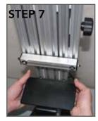
**Step 7: Installing the electric switch** (**DPG1C**) and phone tray. After the base has been attched, prep the tray by unscrewing the e-nuts until they are on the end of the bolt. Slide the tray on using the vertical channels of the lifting assembly as shown. Slide the tray up about 2 inches (this can be changed at any time), and lightly tighten the two bolts with the provided allen wrench.
