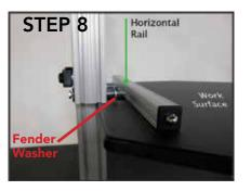
**Step 8:** Lift the Work Surface up and align the holes in the Horizontal Rail with the (2) 1/4-20 x 3.50 Hex Head Bolts{B}. Push the Work Surface onto the Hex Head Bolts until the threads of the bolts come through the Horizontal Rail.
