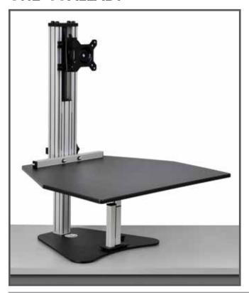
The Wallaby is designed to hold your monitor mounted in a fixed position, and will travel up and down with your keyboard and mouse on the work surface. Your Wallaby is shipped in the down position with the work surface brake tightened. The mount may need adjusted to your desired height for both the seated and standing position.
