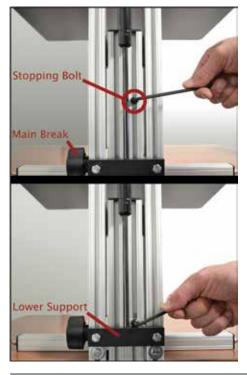
On the back side of your unit you will notice a small bolt located on the lifting tower. This bolt is used as our work surface stopper. It is currently set at 15", the highest our unit should go. This setting is for a 6'2" user on a 30" high desk. If you are shorter than this, raise the unit to your desired height and tighten the Main Brake. Adjust the stopping bolt by loosening the bolt with one turn and drop the bolt down to reach the lower support, and re-tighten the stopping bolt.
